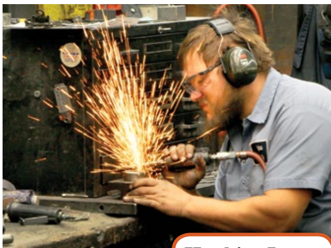
A worker in the Keystone Forging Company grinds finishing touches on a mold.
